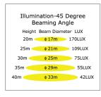
Beam Angle (50% max) 45 DEG Field Angle (10%) **73 DEG** 43,296 lm Luminous Flux (IES) Light Efficacy (IES) 94 lm/W **NEMA Type** 5H x 5V **BUG Rating** B5-U1-G1 UGR 15 **Cutoff Classification** Cutoff
