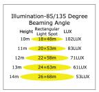
Beam Angle (50% max) 85x135 DEG Field Angle (10%) 130x150 DEG Luminous Flux (IES) 40,813 lm Light Efficacy (IES) 90 lm/W 7H x 7V **NEMA Type BUG Rating** B5-U2-G5 19/32 IES Classification Type II **Cutoff Classification** Semi-Cutoff
